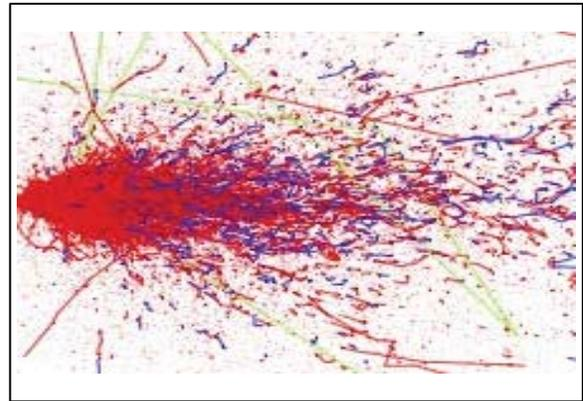
FIGURE 2 - 1000 ELECTRONS AT 50 MEV SIMULATED IN 20 CM OF NaI(Tl) WITH GEANT 4. ELECTRONS ARE IN RED, PROTONS ARE BLUE, AND PHOTONS ARE GREEN.
