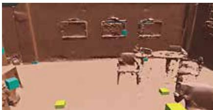
Snapshot of a 3D mesh generated by the Microsoft HoloLens with completed samples (green) and unmarked samples (yellow);
