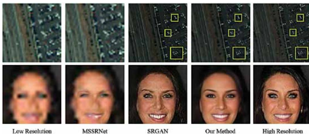
Converting low-resolution images to high-resolution images. The method developed by Dr. Hamid Krim's VISSTA Lab is able to better restore the fine details region (indicated by green boxes) in the high-resolution image.
