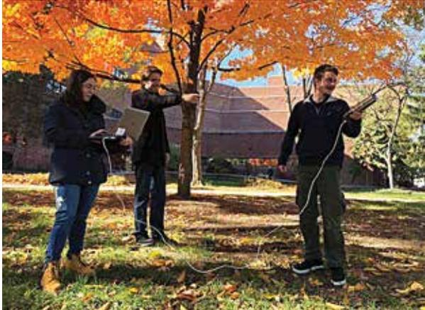
Students work together on campus, to collect urban background measurements, using a sodium iodide (NaI) detector, in order to use them for their ongoing research.
