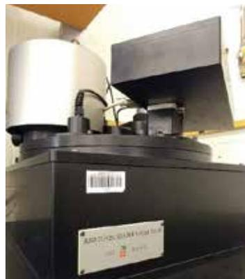
Instrumentation used in this research to measure ubiquitous materials for their integrated dose. On the left is the electron paramagnetic resonance spectrometer and on the right is the combined thermoluminescence and optically stimulated luminescence spectrometer
